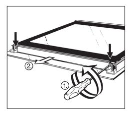
■ Unscrew the Torx screws, and remove the guides, trim and seal.
